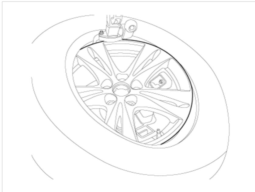
10. Inject air into the tire until the beads are in the correct position.
