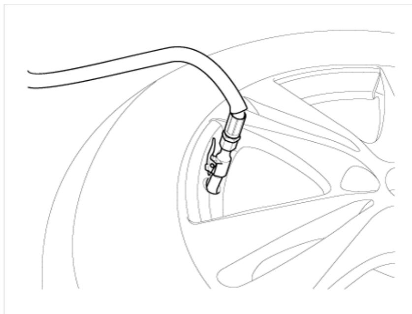
11. Adjust the tire pressure according to the recommended tire pressure for the vehicle.
