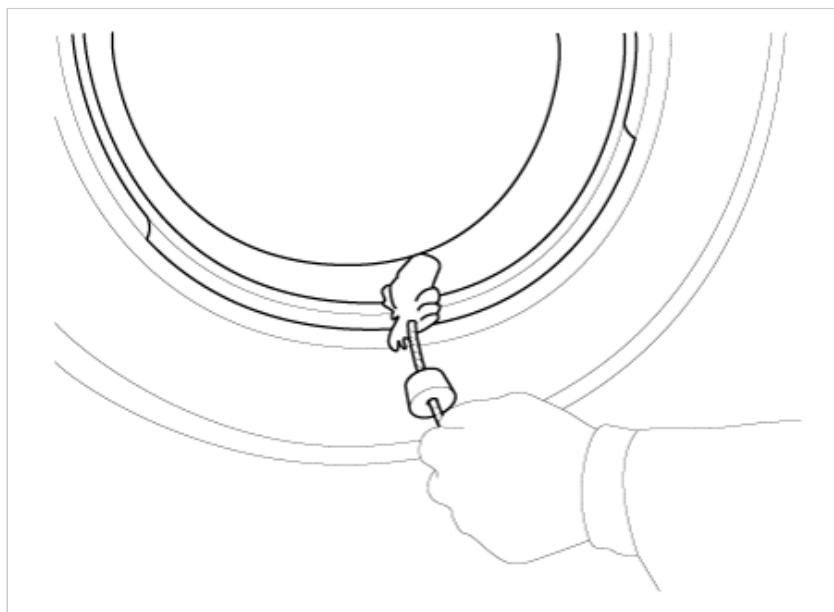
7. In order to mount lower the beads, place the TPMS sensor at 5 o'clock, starting from the head of the tire replacement equipment.
