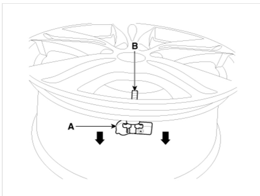
4. Use the valve mounting tool to pull out the valve until it is entirely out of the lower hole.
