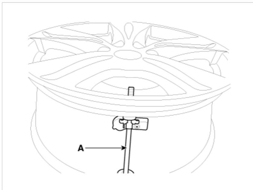
3. Remove the sensor body (A) from the valve (B) in the direction of the arrow.
