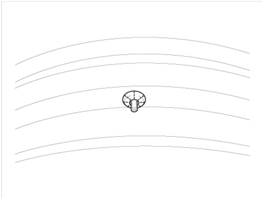
5. Apply lubricant to the surface of the valve, and then mount it through the valve hole of the wheel.
