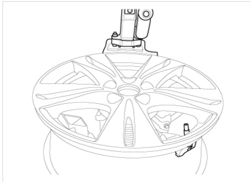
8. Rotate the rim clockwise and press tire towards 3 o'clock to mount the lower beads.
