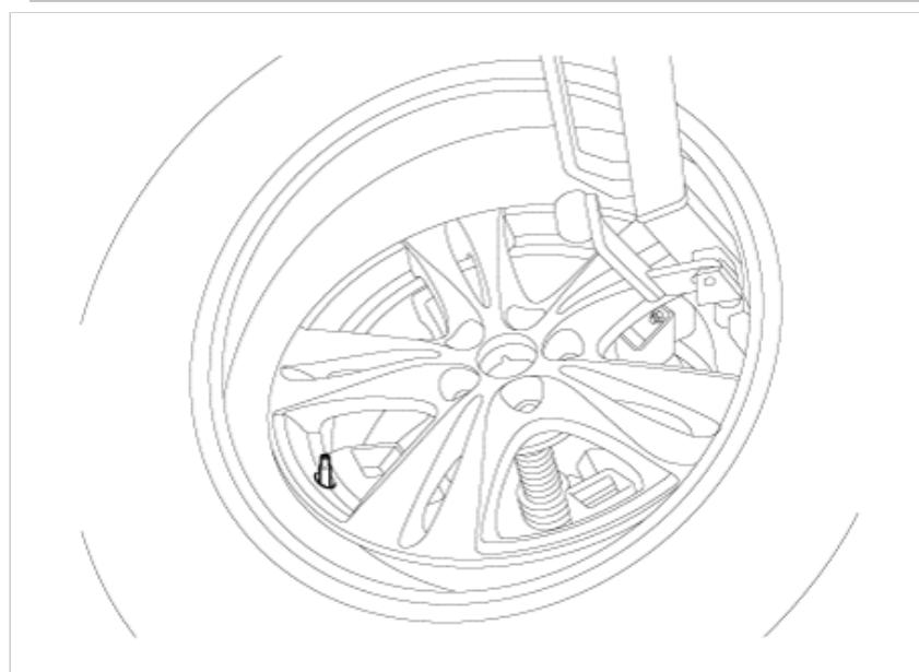
9. In order to mount the upper beads, press the tire towards 3 o'clock and turn the rim clockwise.
